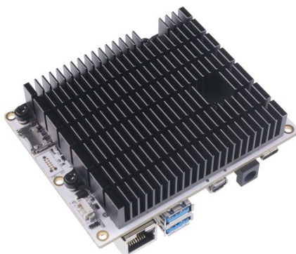
Fig. 6.10: BeagleBone AI-64 back with heatsink at 45° angle
